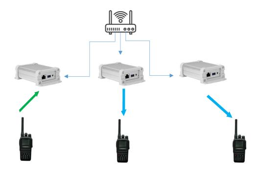
Multiple repeaters (SPECIAL version) can be attached to the LAN. For example, 1 repeater is placed on each floor of a building. When a handset initiates a call, the voice will be transmitted to the entire LAN through the network and forwarded by other repeaters, so as to complete the signal coverage of the entire building. The special feature of this machine is that the entire building can be covered with only one frequency point.
